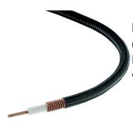
FSJ4RK-50B, HELIAX® Superflexible Foam Coaxial Cable, corrugated copper, 1/2 in, black non-halogenated, fire retardant polyolefin jacket B2ca-sla-dl-al (CPR testing is conducted annually please reference the website for latest classification)
